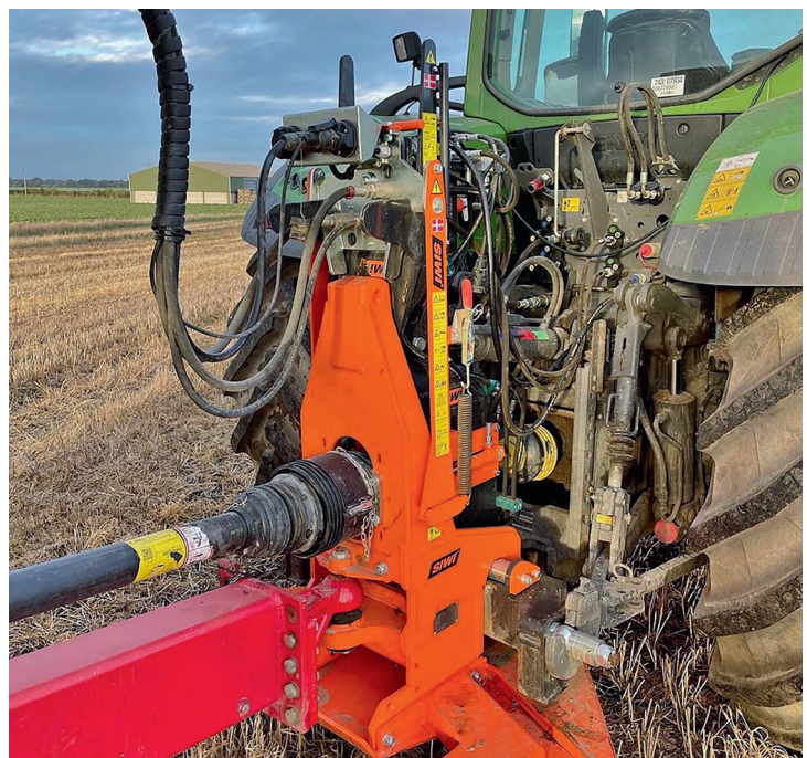
Once the hitch is locked into the drawbar attachment, the operator activates a spool valve which automatically engages the hydraulics, brake, electronics and pto services.
