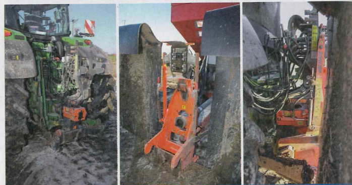
When the trailed spreader is unhitched during loading, the front section of the Combi Hitch remains on the tractor, and the rear section stays with the spreader. When loading is finished, the loader tractor is reconnected to the spreader including the hitch, PTO shaft, Isobus link, five electrical cables and 11 hydraulic hoses in less than five seconds, without the operator leaving the cab.
