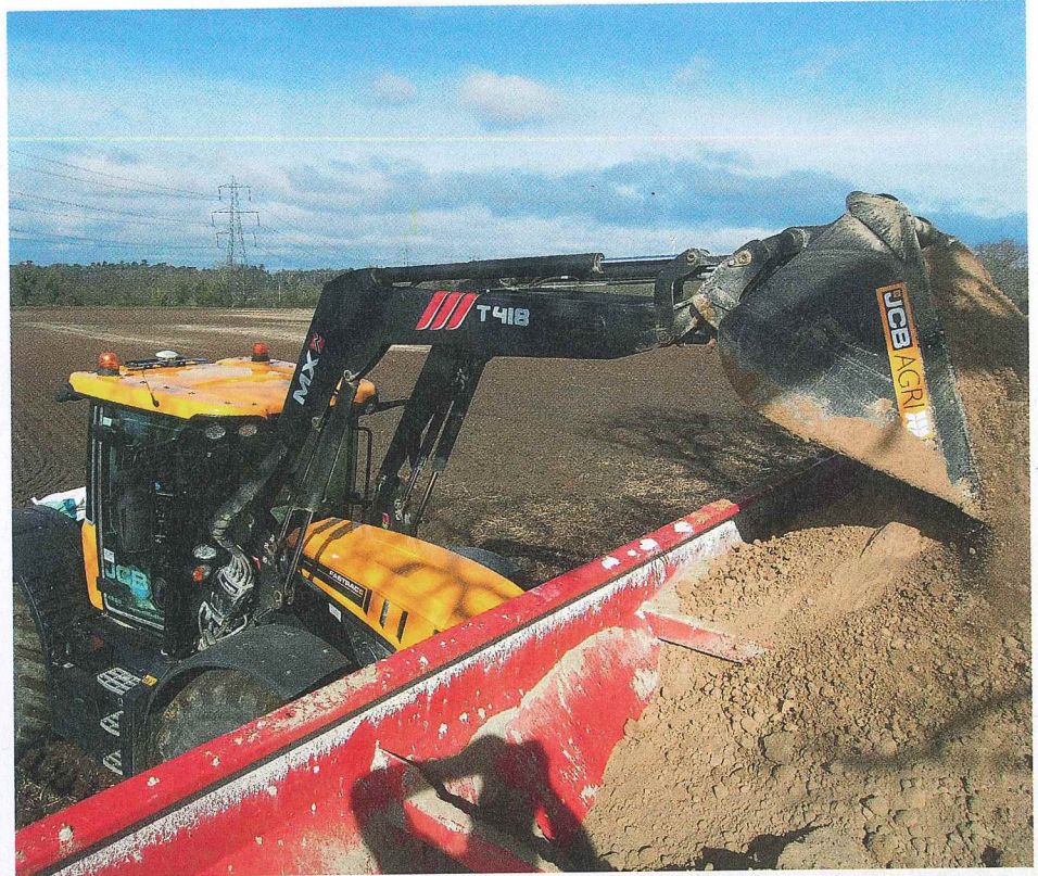
The T418 loader was specified to work with the JCB and offers 3.05 tonnes lift capacity and 4.6m lift height to reach over the side of the high capacity spreader.
