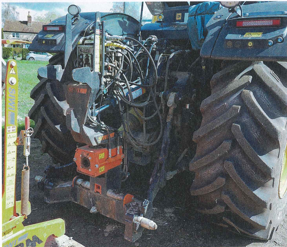
The tractor side - to hitch up, the tractor linkage is lowered, the tractor backed so it is under the trailer frame and then lifted. The hooks engage and lift the drawbar.
