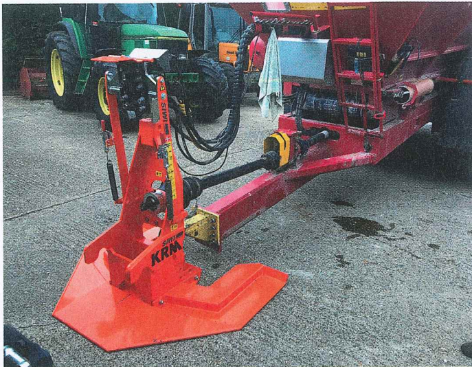
The 'trailer side' of the hitch showing the connections for the pto and hydraulic services, plus the large footplate which supports the spreader while it is being loaded.
