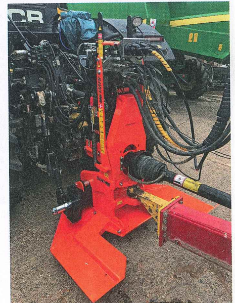
The SiWi hitch connects all services from the tractor to the spreader at once, controlled from the cab.
