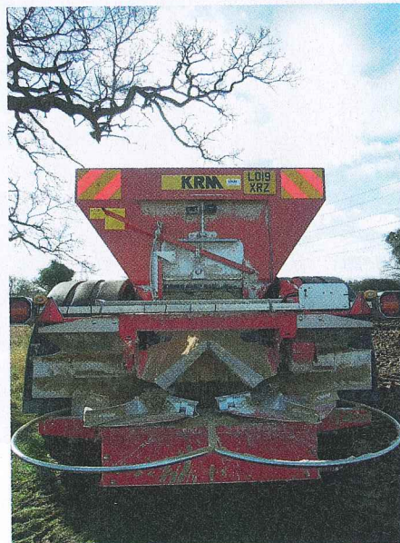
The Bredal K135, imported by KRM, has a capacity of up to 20 tonnes and can spread fertiliser to 24m bouts.
